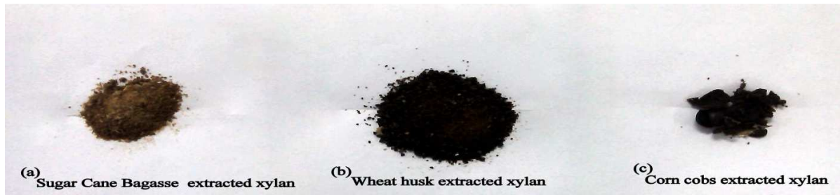
Fig: 2. Dried extracted xylan powders. (a) refers to sugar cane bagasse extracted xylan, (b) for wheat husk and (c) refers to corn cob
